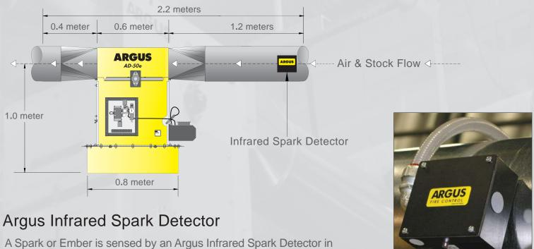
A Spark or Ember is sensed by an Argus Infrared Spark Detector ir 5 milliseconds at speeds up to 60 meters per second.
